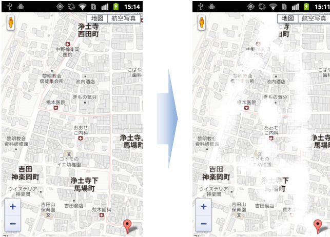
(a) Degrading navigation system (left: a normal map without degradation which is displayed at the beginning, right: a map where the driven route was whitened.)
