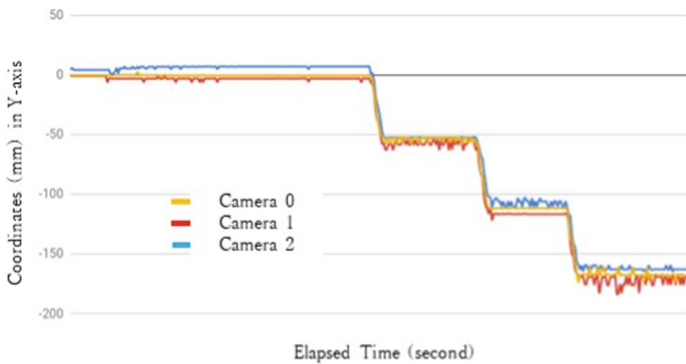
Fig. 22. Coordinates when the single-axis robot is moved in the Y-axis direction by increments of 50 mm. (Color figure online)
