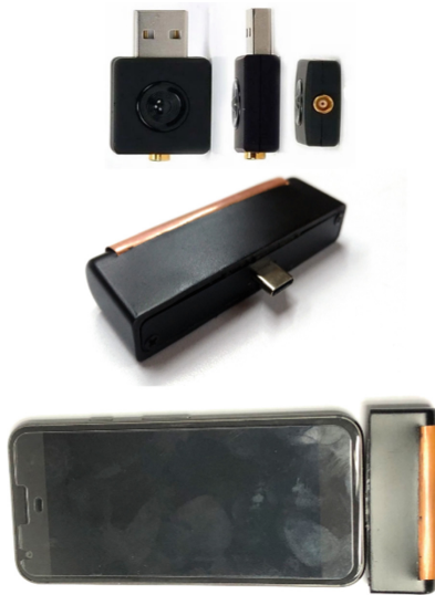
Fig. 2. The original receiver and inner circuit board (left), the modified receiver embedded in the case (mid), and the final attachment coupled with a mobile phone (right)
