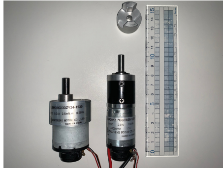
Fig. 3. Two types of DC motors (Left:3254 E_0, Right:3261 E_0) and a their weight.
