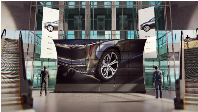
Fig. 1. Overview of the curved public display. This arch-shaped display has a total of 36 ( 6 \times 6 ) 55-in. OLED curved display panels made by LG.
