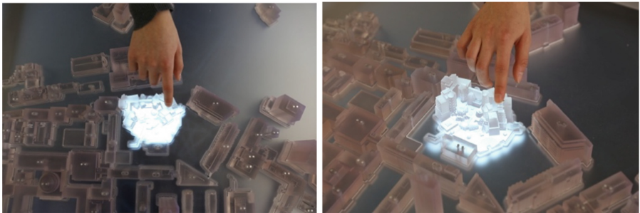
Fig. 3. Photo of user interacting with Tangible Map via touch. Aluminum rods embedded in the 3D printed buildings allow for digital interaction through capacitive charge.
