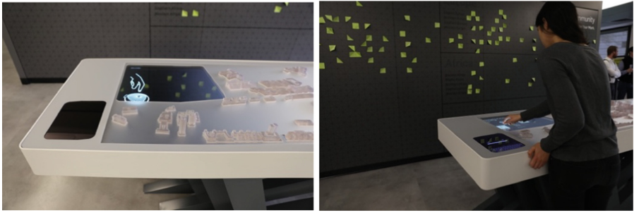
Fig. 2. The Tangible Map consists of two parts; 3D printed buildings to entice users to touch and to provide visual reference, and an interactive tablet that further displays information about the building selected and vice versa.
