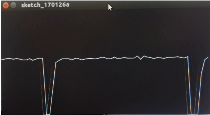
Fig. 2 Graphic plotted by processing program, showing the electric signals sent by bicycle through Arduino to the computer.
