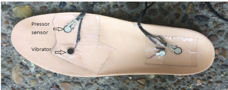
Fig. 4. Sensor implementation at insole
