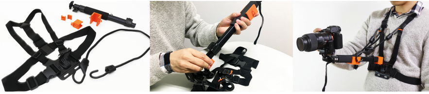
Fig. 2. Left: All of parts we prepared. They consists of a monopod, harness, bungee code, and 3D-printed components. Center: assembly phase of these parts. Right: the user is equipped with our instrument.
