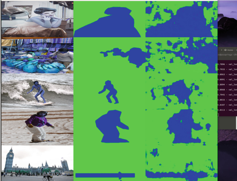
Fig. 9. Showcases very hard validation examples of the image segmentation process. Input images are shown in column 1, the ground truth labels in column 2, and the neural network results in column 3. Background pixels are represented in green, while pixels belonging to people are represented in blue. (Color figure online)
