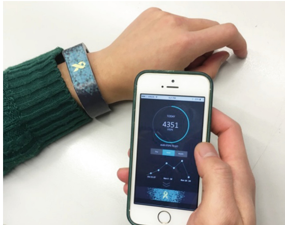
Fig. 5. The prototype of the wrist-worn device and the mobile application of i-Ribbon (non-functional simulation).
