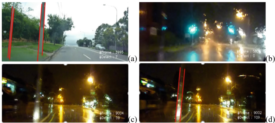
Fig. 4. The results of information filter: (a) sunny day, (b) rainy day, (c) result without filter and (d) result with filter.
