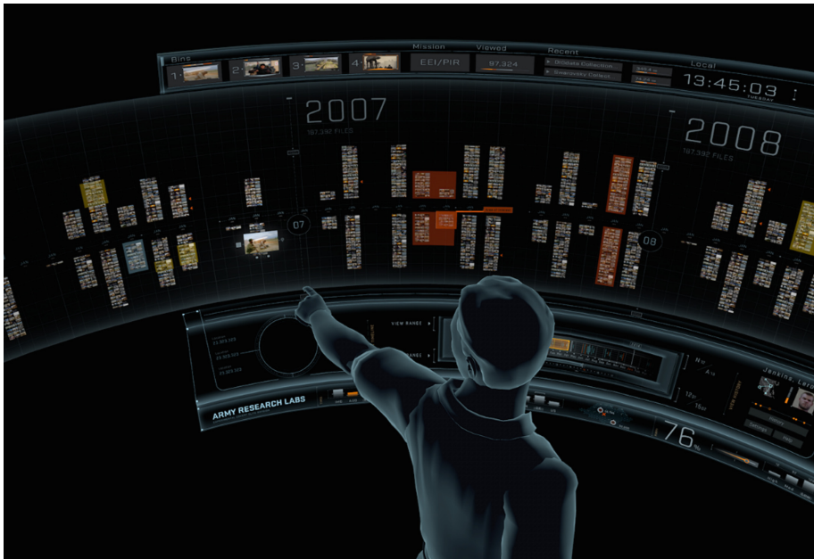
Fig. 1. Over-the-shoulder view of the VIE and a user viewing a photo collection based on time. The timeline graph shown can be zoomed in to see that each part of the graph is composed of the images taken during that part of the timeline. The images are framed on the top and bottom by the non-moving VIE console.
