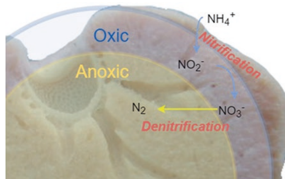
Fig. 9.3 Simplified diagram of nitrification and denitrification superimposed on a vertical slice of a sponge Geodia barretti
