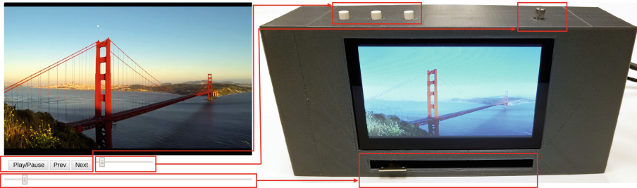
Fig. 4. Video Player: At left, a demo of a video player which provides a familiar on-screen interface for playing videos. At right, Amalgam allows the same demo to drive a fully-tactile interface, the only difference being the style sheet.
