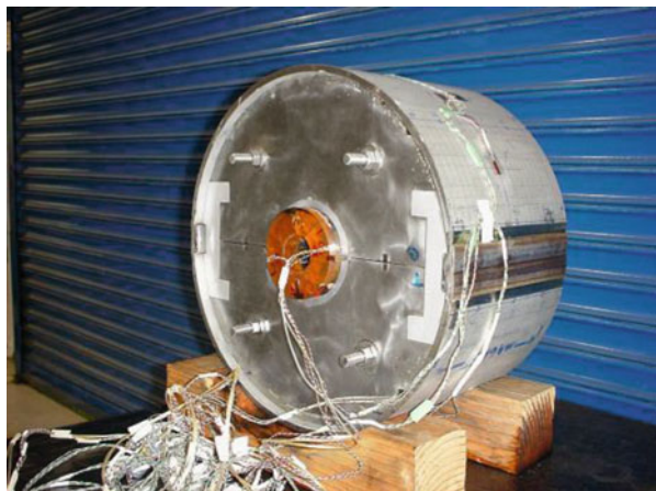
Fig. 7.6 Instrumented short mechanical model. (Andreev et al. 2000)
