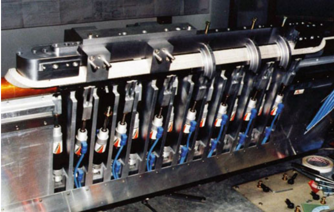
Fig. 4.10 Winding a coil layer. (Courtesy of ELIN, Austria)
