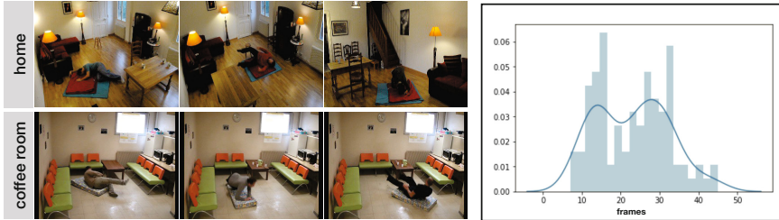
Fig. 3. From left to right: (1) Sample frames of falls in home and coffee room . (2) The statistics of time durations of falls across all videos, in which the x-axis denotes the fall duration, the y-axis and the bins show the normalized occurrence frequencies and the curve shows the fitted distribution.
