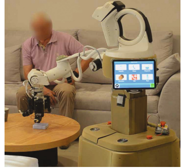
Fig. 1. The RAMCIP robot engaged on a medication assistive task.
