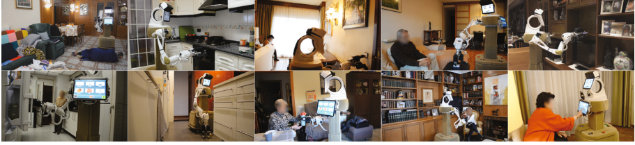
Fig. 8. Examples of RAMCIP interacting with users and the environment during the preliminary trials. Top row: SU1.1 (emergency), SU2.1 (turning off electric appliances), SU2.2 (turning on the light), SU2.3 (detection of improperly place objects), SU3.1 (medication bringing). Bottom row: SU4.1 (assistance upon detection of abnormalities during cooking), SU4.2 (assistance for fallen objects), SU5.1 (proactive bringing bottle of water), SU5.2 (on demand bringing a snack), SU6.1 (provision of cognitive training).
