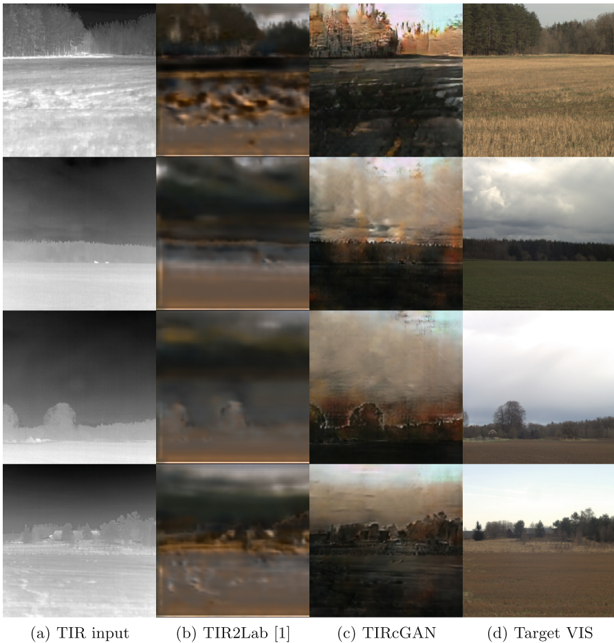
Fig. 5. Examples for methods output when trained on the KAIST-MS dataset [4] and evaluated on the FOI dataset. Both models struggle with predicting the colors since the two datasets were captured in different environments. However, TIRcGAN can still predict the objects in the scene.
