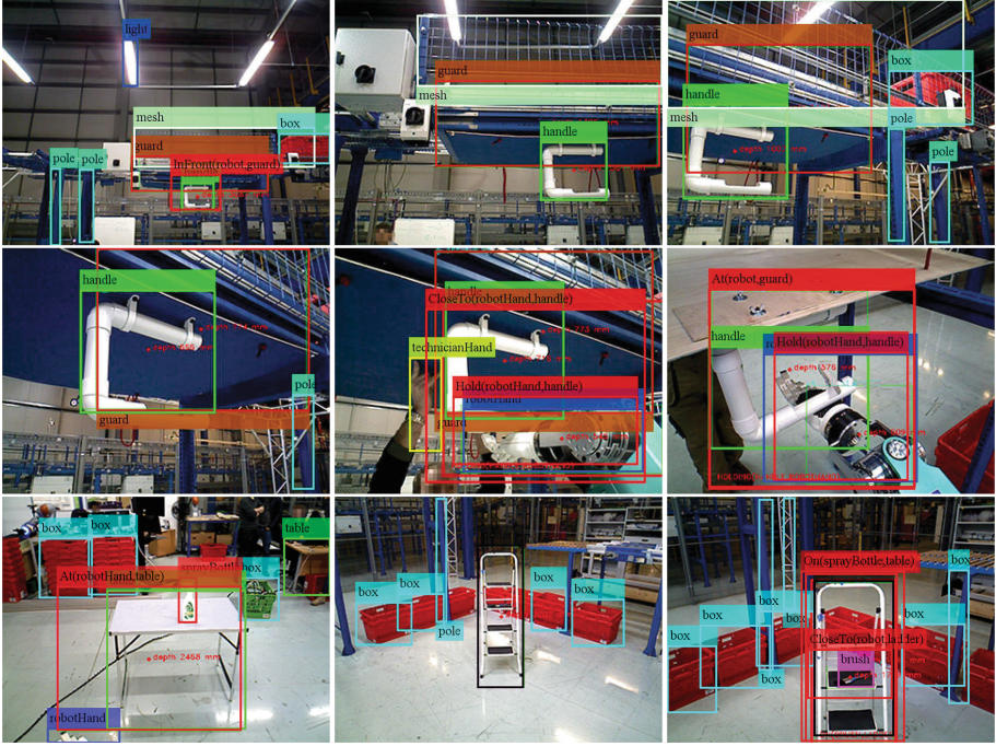
Fig. 4. Recognition during tasks execution. The sequence shows the detection of guard (panel), handle and its manipulation to lower it helping the technician to hold the guard for inspecting the rollers. The involved relations are At , Hold , InFront , On , and CloseTo .
