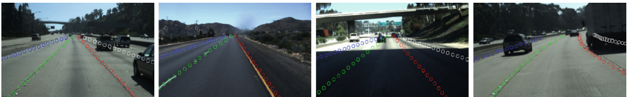
Fig. 1. Example of multilane detection and classification by our network, where the output is in the form of lane boundary image coordinates represented by small color circles (best viewed on computer screen when zoomed in). Classified leftside , leftego , rightego and rightside lane boundaries are represented by blue, green, red and white colors respectively (best seen in color) (Color figure online)
