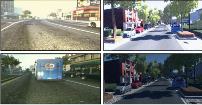
Fig. 4. Example augmentations of GTA (left column) and VKITTI (right column) using the proposed sensor effect augmentation pipeline. Each image has a randomly sampled level of blur, chromatic aberration, exposure, sensor noise, and color temperature shift applied to it in an effort to model the visual structure/information loss caused by cameras when capturing real images.
