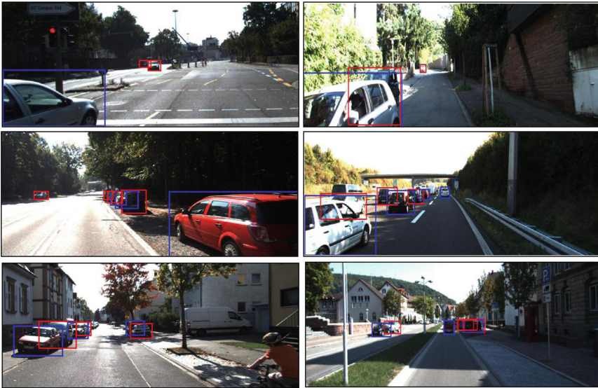
Fig. 5. Virtual KITTI examples are in the left column, GTA examples are in the right column. Blue boxes show correct detections; red boxes show detections missed by the FasterRCNN network trained on baseline, unaugmented image datasets but detected by FasterRCNNs trained on data augmented using our proposed approach for sensor-based image augmentation. (Color figure online)
