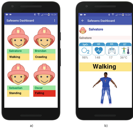
Fig. 2. Screenshots of the team leaders' application showing (a) the dashboard, and (b) the screen with details of the current HAR estimate.
