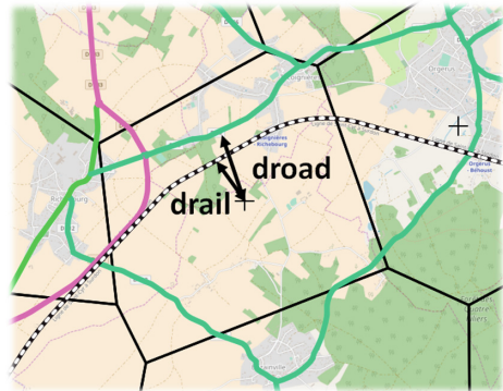
Fig. 2. Example of a voronoï sector and its associated shortest distance to transports axes. Five roads (colored lines) and one rail line (dashed line) intersect the sector. (Color figure online)
