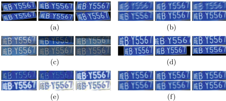
Fig. 3. Six data augmentation methods (a) Affine transformation (b) Motion blur (c) Uneven light (d) Stretching transformation (e) Erosion and dilation (f) Down sampling and gaussian noise.
