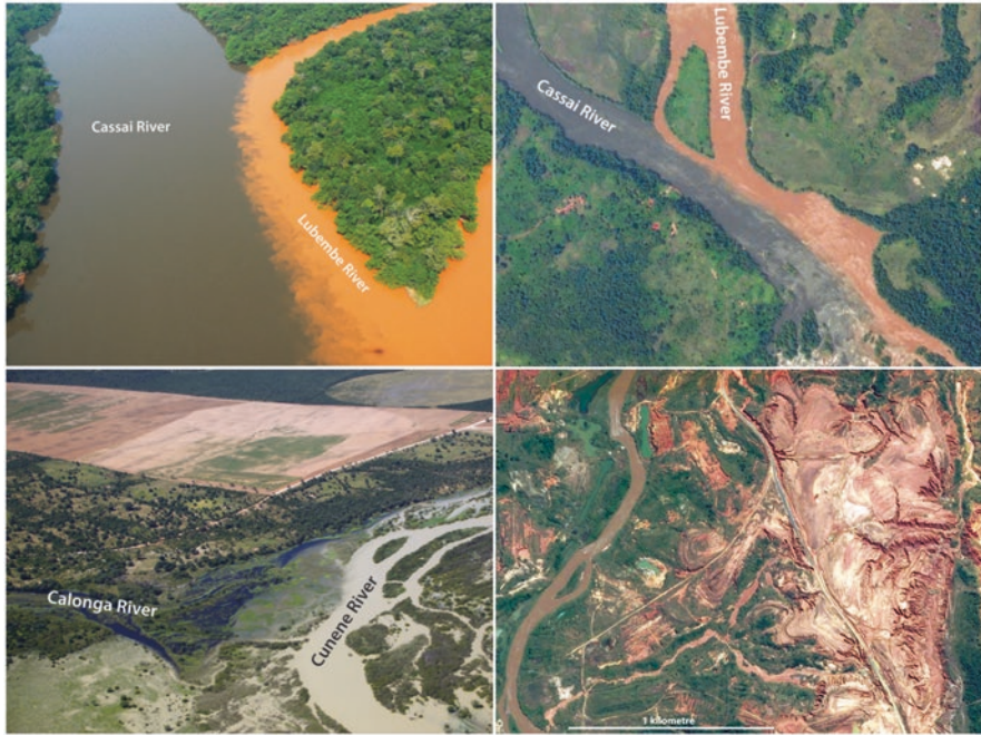
Fig. 8.5 Mining impacts on Angolan rivers. Top left and right: The confluence of the clear Cassai River and the turbid Lubembe River carrying suspended sediments from open-cast diamond mining in Lunda-Norte. The confluence is in the DRC about 80 km north of Angola’s border. The left photograph was taken on 30 May 2007, while the right image from Google Earth was taken 10 years later on 21 May 2017, viewed from 6.62 South, 21.07 East. Bottom left: The confluence of the Calonga and Cunene rivers at Quiteve (16.02 South, 15.20 East), showing the volumes of eroded sediments from upstream in the Cunene catchment. By contrast, the clear waters of the Calonga mainly come from areas where arenosols predominate, where few people live and where large areas of woodland have not been cleared for dryland agriculture. Bottom right: Erosion from open-cast mining along the Luachimo River 22 km north of Lucapa. (The image from Google Earth was taken in May 2017 as viewed from 8.23 South, 20.77 East)
