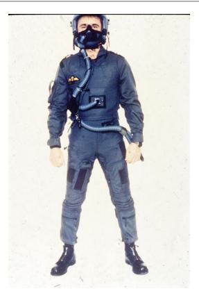
**Fig. 3** Representative Positive Pressure Breathing Ensemble. Picture shows the helmet/oronasal mask, thoracic jerkin, anti-G suit, and connectors/tubing. The breathing system is tied into the aircraft's life support breathing supply and regulator (blend of bottled  $O_2$  and engine bleed air). Reproduced with permission from the Canadian Department of National Defence. The source is Defence R&D Canada
