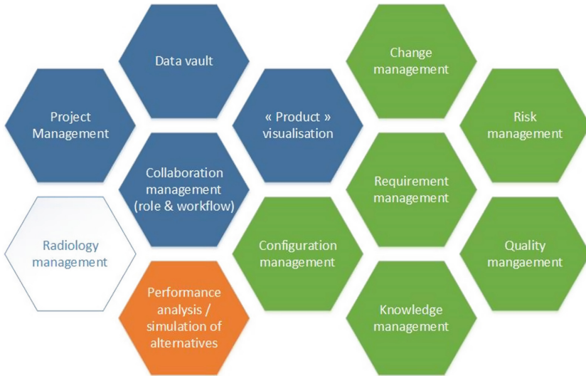
Fig. 2. BIM-PLM functionalities elicited for NFD: in green PLM-specific functionalities, in red BIM-specific ones, in blue BIM-PLM common ones and in white NFD-specific one. (Color figure online)
