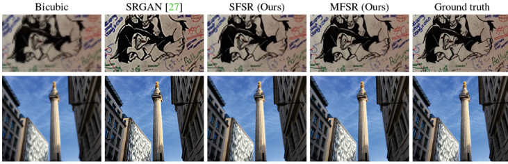
Fig. 8. Multi-frame 4\times super-resolution on stabilized Live Photo test data. While our single frame model achieves a good upsampling, the increase in sharpness from our multi-frame approach brings a significant quality improvement.
