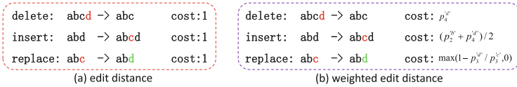
Fig. 5. Illustration of the edit distance and our proposed weighted edit distance. The red characters are the characters will be deleted, inserted and replaced. Green characters mean the candidate characters. p_{index}^c is the character probability, index is the character index and c is the current character. (Color figure online)
