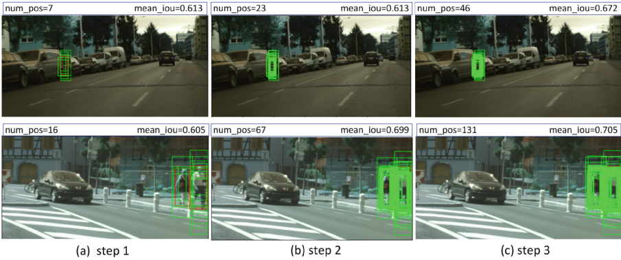
Fig. 2. Two examples from the CityPersons [44] training data. Green and red rectangles are anchor boxes and groundtruth boxes, respectively. Values on the upper left of the image represent the number of anchor boxes matched with the groundtruth under the IoU threshold of 0.5, and values on the upper right of the image denote the mean value of overlaps with the groundtruth from all matched anchor boxes.
