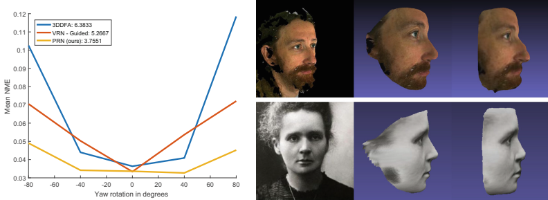
Fig. 9. Left: CED curves on Florence dataset with different yaw angles. Right: the qualitative comparison with VRN-Guided. The first column is the input images from Florence dataset and the Internet, the second column is the reconstructed face from our method, the third column is the results from VRN.
