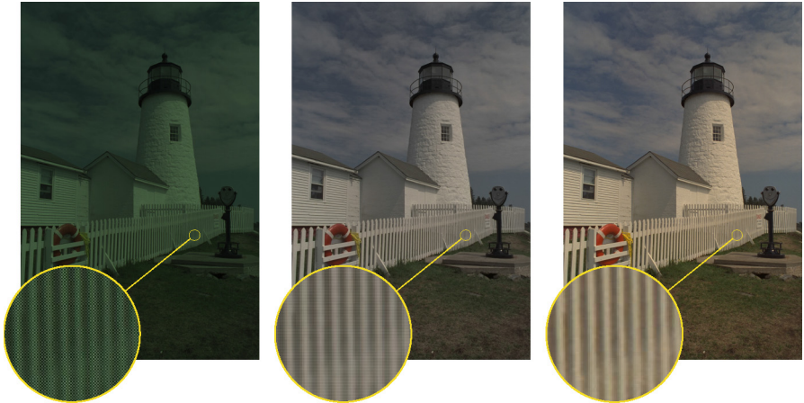
Fig. 2. Progression along the steps of our demosaick network. The first image which corresponds to Step 1 represents a rough approximation of the end result while the second (Step 3) and third image (Step 10) are more refined. This plot depicts the continuation scheme of our approach.
