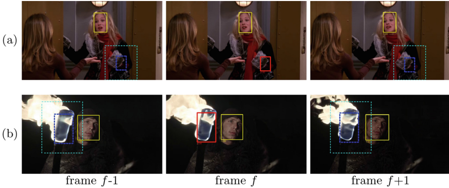
Fig. 2. Mining hard negatives from detector-flicker. The solid boxes denote detections, and the dashed boxes are associated with the tracking algorithm. Given all of the high-confidence face detections in a video ( yellow boxes), the proposed algorithm generates a tracklet ( blue dashed boxes) for the current detection ( red box in frame f ) by applying template matching within the search regions of the adjacent frames ( cyan dashed boxes). As there are no matching detections in adjacent frames for the current detection ( i.e. no yellow box matches the blue dashed boxes in frames f - 1 or f + 1 ), it is correctly considered to be an “isolated detection” and added to the set of hard negatives . The remaining detections in frame f , which are temporally consistent, are added to the set of pseudo-positives . (Color figure online)
