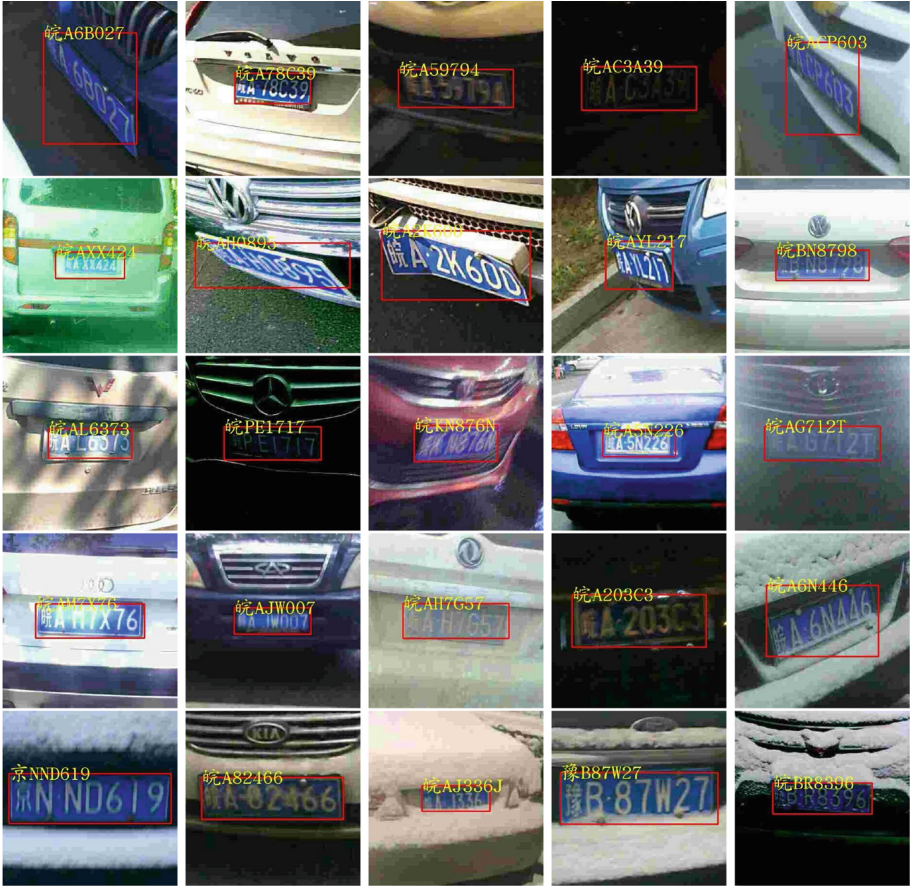
Fig. 4. Detection and recognition results on CCPD with our RPnet model. Each image is the smaller license plate area extracted from the original resolution 720 (Width) \times 1160 (Height) \times 3 (Channels).
