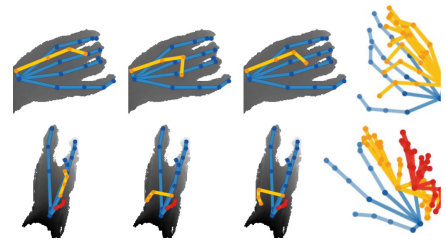
Fig. 3. Hand images under self-occlusions exhibiting multiple pose labels.
