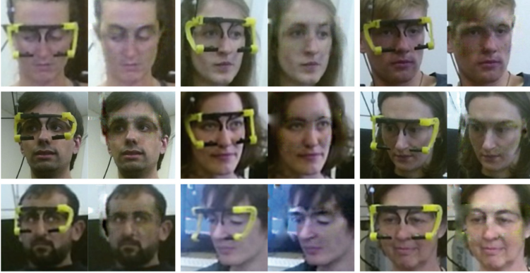
Fig. 6. Image pairs showing the original images of the subject wearing the eyetracking glasses (left) and the corresponding inpainted images (right). The inpainted images look very similar to the subjects’ appearance at testing time and are thus suited to train an appearance-based gazed estimator. Figure best viewed in color.
