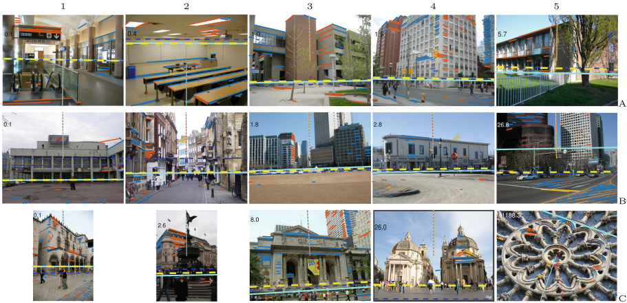
Fig. 4. Horizon lines obtained at the 1st, 25th, 50th, 75th and 100th percentiles of the horizon error (Col. 1–5, resp.) for YU (Row A), EC (Row B) and HLW (Row C). The GT HL is shown in yellow dashed line, the MMMs in blue dashed lines and the estimated HL in cyan solid line. The horizon error is displayed on the top-left corner of each image result. LSs participating to a VP are shown using one color per VP. (Color figure online)
