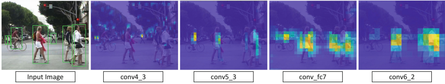
Fig. 2. Visualization of feature maps from different convolutional layers. Shallow layers have strong activation for small size targets but are unable to recognize large size instances. While deep layers tend to encode pedestrians of large size and ignore small ones. For clarity, only one channel of feature maps is shown here. Best viewed in color.
