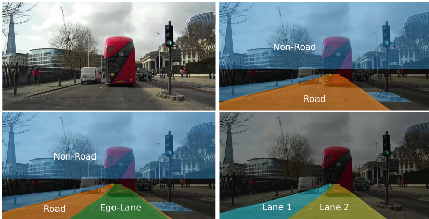
Fig. 1. Example image from our dataset (top left), including annotations for road (top right), ego-lane (bottom left) and lane instance (bottom right). Road and lanes below vehicles are annotated despite being occluded. Non-coloured parts have not been annotated, i.e. the class is not known.
