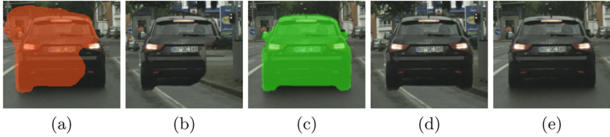
Fig. 1. Learning to Segment by Cut and Paste. We iterate to learn accurate segmentation masks by trying to generate realistic images. A poor mask estimate (a) generates an unconvincing paste (b), while a good mask (c) results in a convincing one (d). Training a discriminator network to distinguish pasted from real images (e) creates a learning signal that encourages the generator to create better segmentations.
