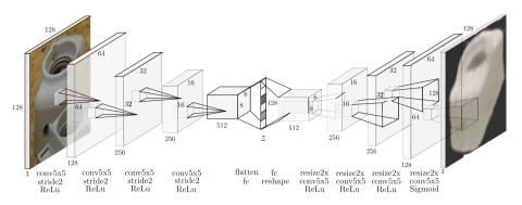
Fig. 5. Autoencoder CNN architecture with occluded test input
