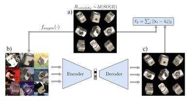
**Fig. 4.** Training process for the AAE; (a) reconstruction target batch  $\boldsymbol{x}$  of uniformly sampled SO(3) object views; (b) geometric and color augmented input; (c) reconstruction  $\boldsymbol{\hat{x}}$  after 30000 iterations
