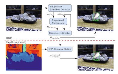
Fig. 1. Our 6D object detection pipeline with homogeneous transformation  $H_{cam2obj} \in \mathbb{R}^{4x4}$  (top-right) and depth-refined result  $H_{cam2obj}^{(refined)}$  (bottom-right)
