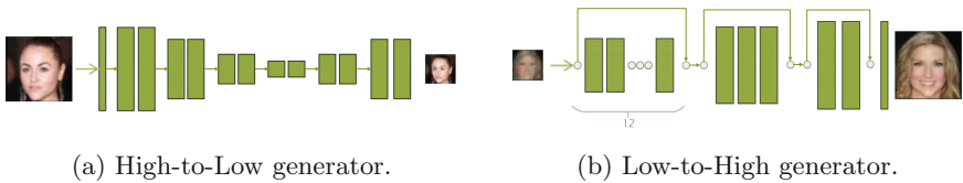
Fig. 4. The generator architecture used for the (a) High-to-Low and (b) Low-to-High networks. The residual block used is shown in Fig. 6b.
