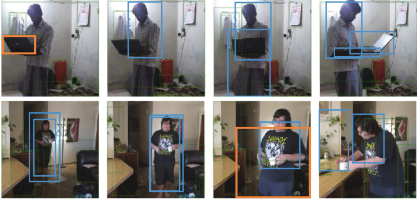
Fig. 3. Similarity Graph \mathbf{G}^{sim} . Above figure shows our similarity graph not only captures similarity in visual space but also correlations (similarity in functional space). The query box is shown in orange, the nearest neighbors are shown in blue. The transparent green boxes are the other unselected object proposals. (Color figure online)
