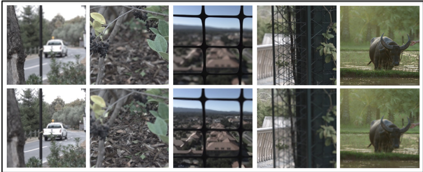
Fig. 6. The performance of our two-stage refocusing framework on generic images. The first row has the input wide-aperture image and the second row shows the refocused image. The first four columns show the performance on structurally different light-field focal slices from another light-field dataset while the last column shows the performance on an image captured by a wide-aperture camera.
