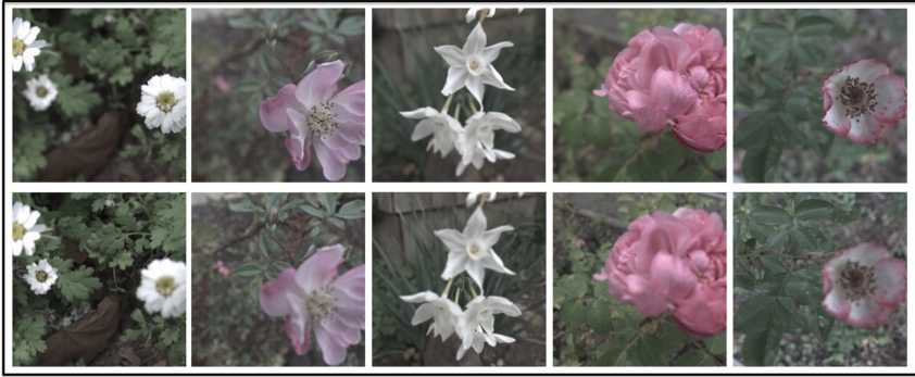
Fig. 8. Near-to-Far Refocusing generated with \delta = +9 using our refocusing network. The top row shows the input wide-aperture images and the bottom row shows the output refocused images.
