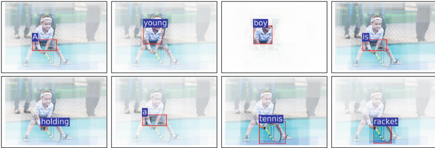
Fig. 4. Visualization of the attended image regions with respect to each word in the sentence description, outlining the region with the maximum attention weight in red. The regional brightness represents the attention strength, which considers the importance of both region and word estimated by our model. Our model generates interpretable focus shift and stresses on words like “boy” and “tennis racket”, as well as the attributes (young) and actions (holding). (Best viewed in color) (Color figure online)
