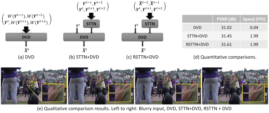
Fig. 8. Comparisons with DVD [45]. A function W in (a) warps the target frame to the reference frame.
