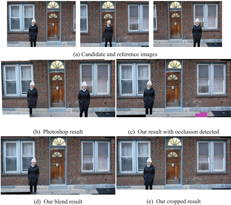
Fig. 10. Three image stitching. In (c), we choose to not use the human in the right-most input. However, the legs block any information regarding the sidewalk, making this location occluded. Our algorithm correctly labels it as occluded and colors it magenta. (d) and (e) present ways to fix this occlusion. (Color figure online)
