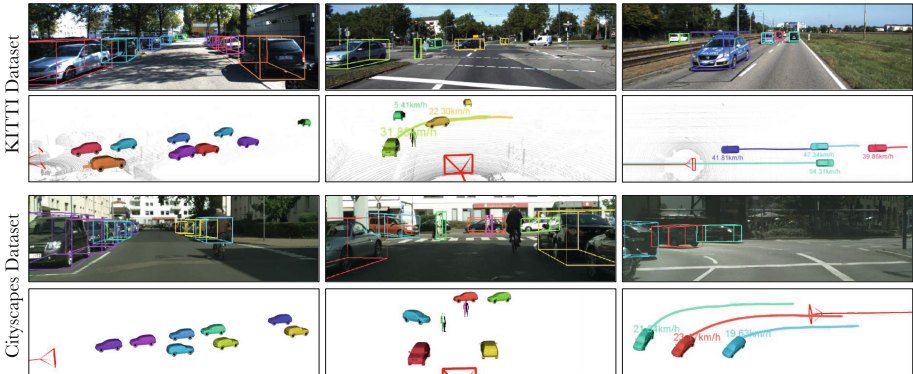
Fig. 7. Qualitative examples over diverse scenarios. From left to right: Concentrated cars. Crossroads which include both cars and pedestrians (note that we do not solve orientation for pedestrians), Dynamic cars. The top two rows are the results on the KITTI dataset, and the bottom two rows show the results on the Cityscapes dataset.
