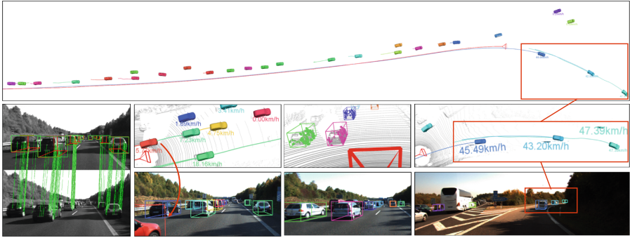
Fig. 1. Overview of our semantic 3D object and ego-motion tracking system. Top: 3D trajectories of ego-camera and all objects in the long travel history. Bottom: from left to right: stereo feature matching for each object (Sect. 5). An extreme car-truncated case where our system can still track the moving car accurately. Dynamic 3D sparse feature recovered by our object BA. Consistent movement and orientation estimation.
